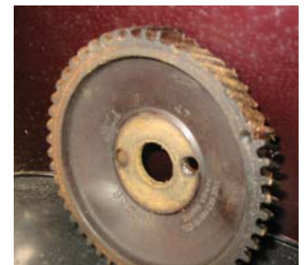
Hansel's timing gear was the culprit. JB Weld could not restore this one!
