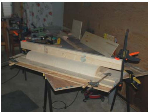
Key to ascetics as well as to aerodynamics is the genteel radius on the rear edge of the lid. Here is Keith's exquisite panel bending jig.
